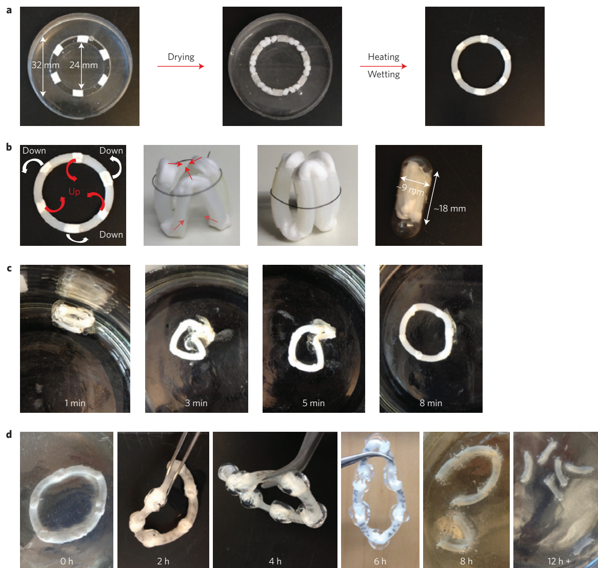
Figure 3 | Construction of a ring-shaped gastric-retentive device and in vitro testing of its elasticity and enteric property. a , Construction of a circle composed of polycaprolactone (PCL) arcs with intervening EE polymer gel linkers by first fitting cubic polymer gels and PCL beads alternately in a circle-shaped polydimethylsiloxane (PDMS) mould, followed by melting PCL at 70 °C. b , Folding of the ring into a standard gelatin 000 capsule by using the elasticity of the polymer gel. c , Escape from the capsule and recovery to the ring shape after dissolution of the gelatin capsule in SGF at 37 °C. d , Progressive dissolution of the EE supramolecular polymer gel linkers in SIF at 37 °C leads to for the dissociation of the circle-shaped device into PCL arcs.
